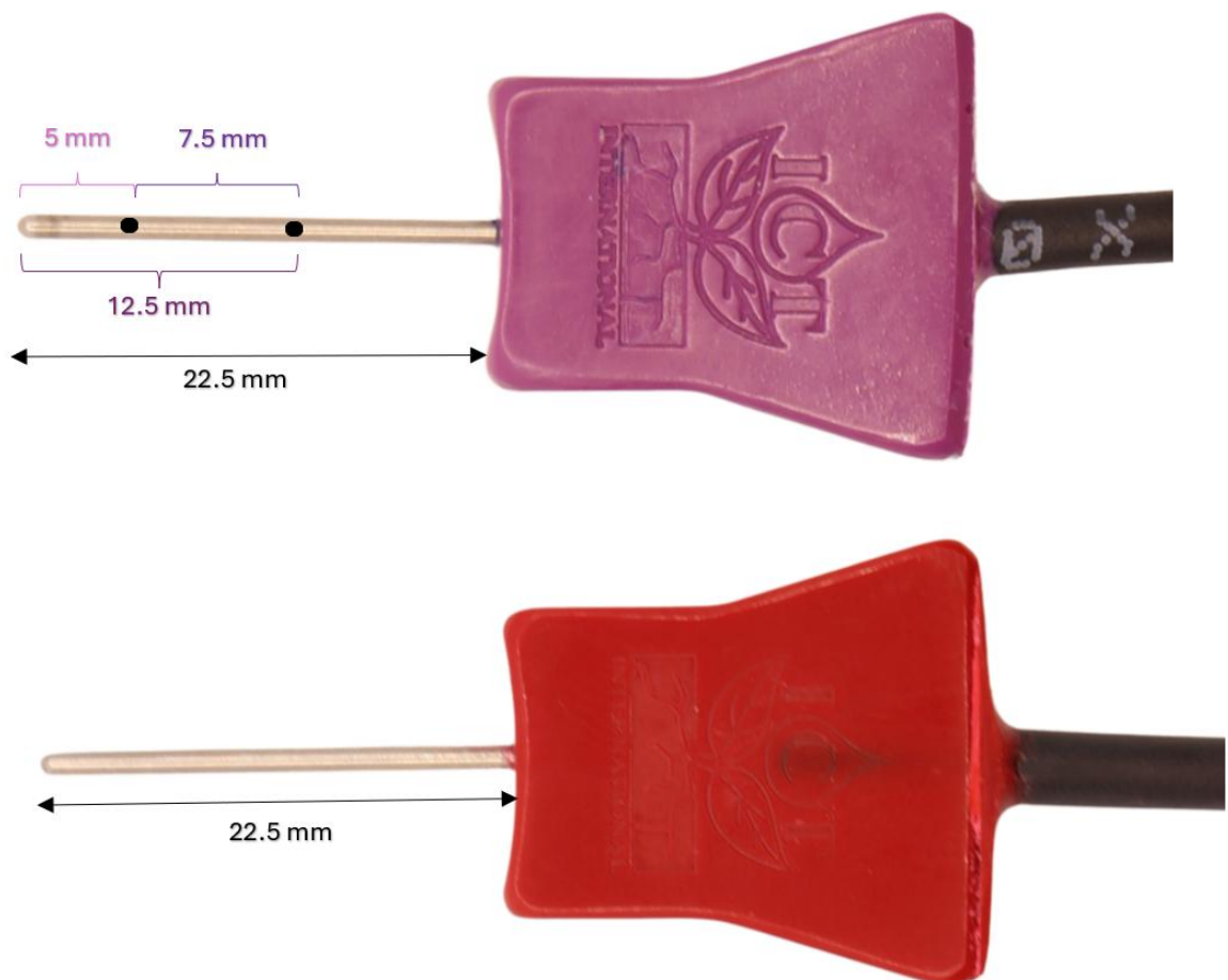
Figure 1.2.1: "SF22.5-TP" 22.5mm length thermistor probe – thermistors position and 1 "SF22.5-HP" 22.5mm length constant current heater
