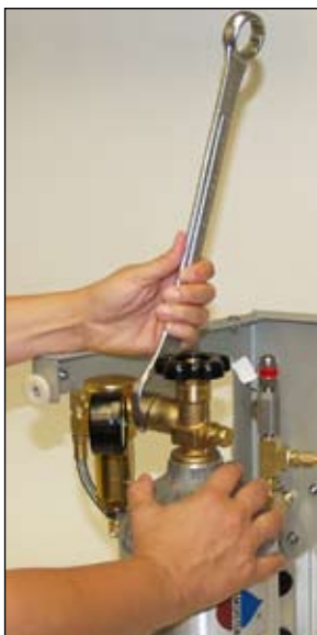
Fig. 16 - Removing the tank by loosening the bolt.
