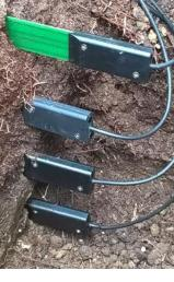
Install sensors addressed 0 closest to the surface, with the highest number being the deepest probe. Sensors numbers are labelled on the cable at both the Node and Sensor ends.
