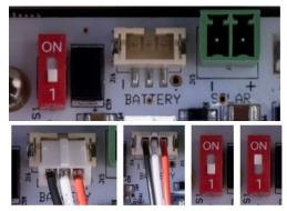
3. After the node is powered via the internal battery connect the solar panel plug
