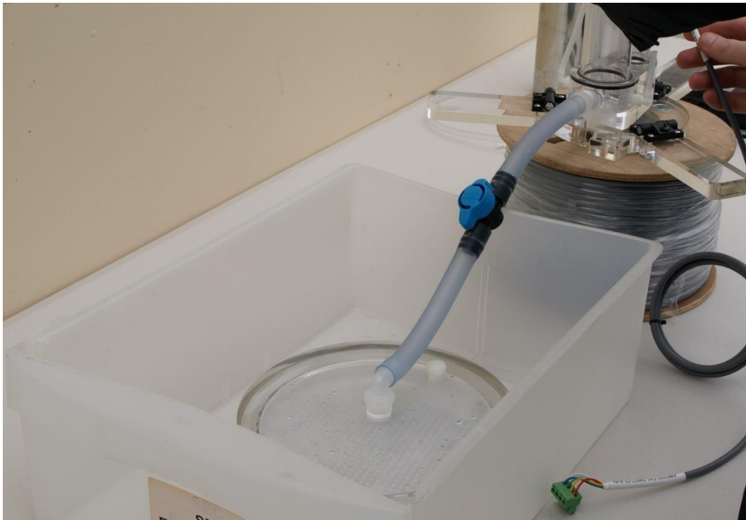
Infiltrometer tower placed on a raised level surface, with the plate below the level of the tower.
