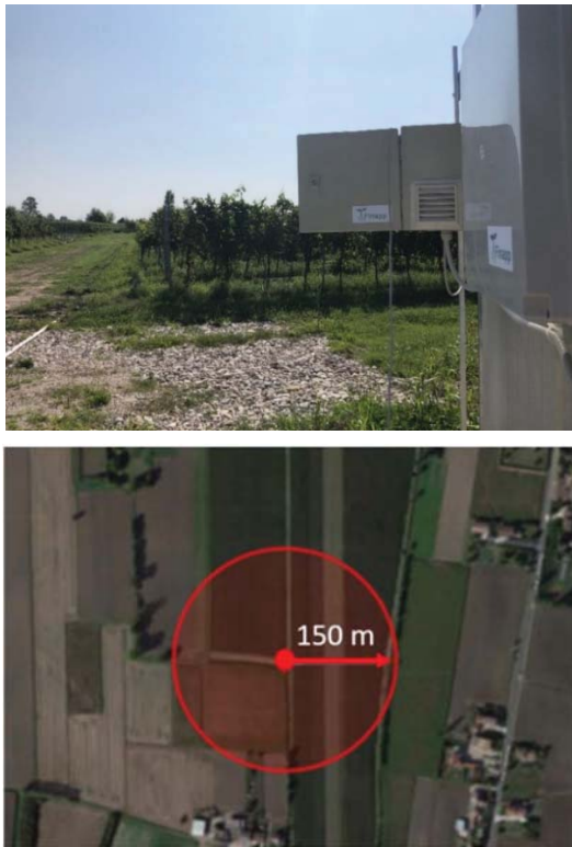
Fig. 4. (upper picture) CRNS-Finapp probe installed at Casalserugo, Padova - Italy; (lower map) the experimental agricultural fields and the effective radius (150 m).
