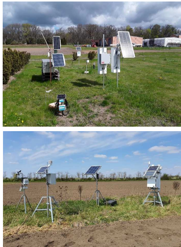
Fig. 1. Experimental sites showing the CRNS sensors (top) at Marquardt site, and (bottom) at Vienna site.
