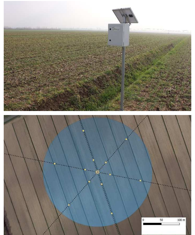
Fig. 3. Ceregnano experimental site, with (above) CRNS-FINAPP and (bottom) soil sampling locations and CRNS footprint (150 m radius).
