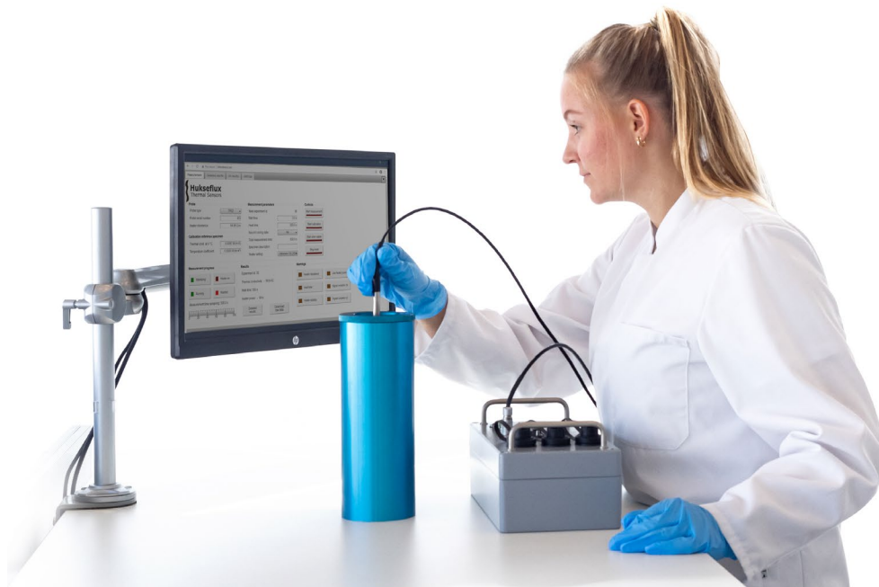
Figure 0.1 Application of the complete TPSYS20 measuring system in a laboratory environment using a CRC01 calibration reference cylinder
