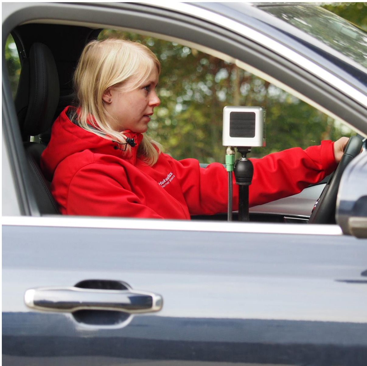
Figure 0.4 TCOM01 applied in car passenger comfort testing
