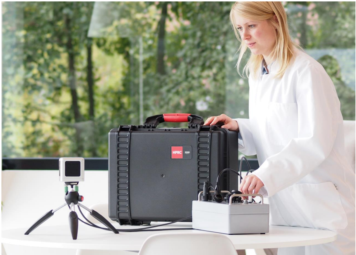
Figure 0.3 A complete system for measuring thermal comfort
