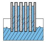
This term refers to those materials, such as porous ceramics and metals, that have a natural ability to fill pores by capillary action. This means the pores and channels of a ceramic have a highly charged pore surface that attracts and bonds the polar molecules of water and other polar fluids. The net effect is called "wicking" --- the ability to pull fluids into the material and transport that fluid by capillary forces. Soilmoisture ceramics are all hydrophilic.
