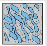
As the name would imply, this is a material in which the pathways or channels are blocked and do not provide the fluid a continuous and interconnected network of channels to connect one surface of the material to an opposing surface.
