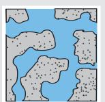
An open pore structure denotes a material that permits a fluid to move from one surface to an opposing surface in the material through a convoluted pathway of interconnecting networked channels. Soilmoisture ceramics are an example of an open pore structured material.
