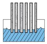
This term refers to materials such as porous plastics that have no affinity to wetting by water. These substances may have pores and channels but have no surface ability to wick water into the pores by the action of capillarity. Such materials are generally made from long chain organic molecules which have no substantial surface charges. Without a charged surface, there is no attractive or bonding effects on the polar molecules of water, and such substances must be specially treated.
