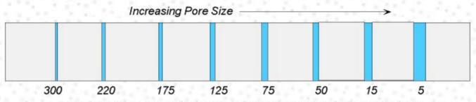
Pressure differential necessary to "break through" the wetted pore in psi
