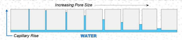
Once wetted by water, the pores within the ceramic will wick water up the interior, filling the pore to differing lengths based on their size.
