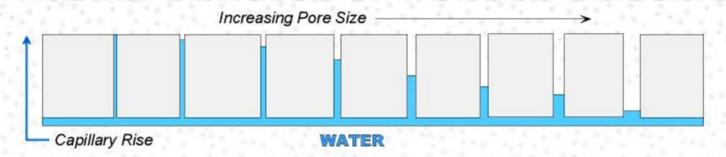
The smaller the pore diameter the better the wicking action (Capillary Rise). Once filled with water the pores provide a liquid interface for measuring and monitoring adjacent other water filled media such as a soil.
