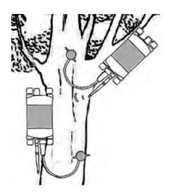
When the PSY logger is installed in the field, ICT International recommend the following mounting methods to increase water repelling action.
