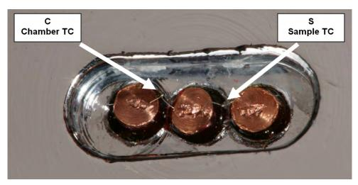
**Photo:** 25 µm Chromel/Constantan thermocouples viewed under a dissection microscope at 20X magnification.
