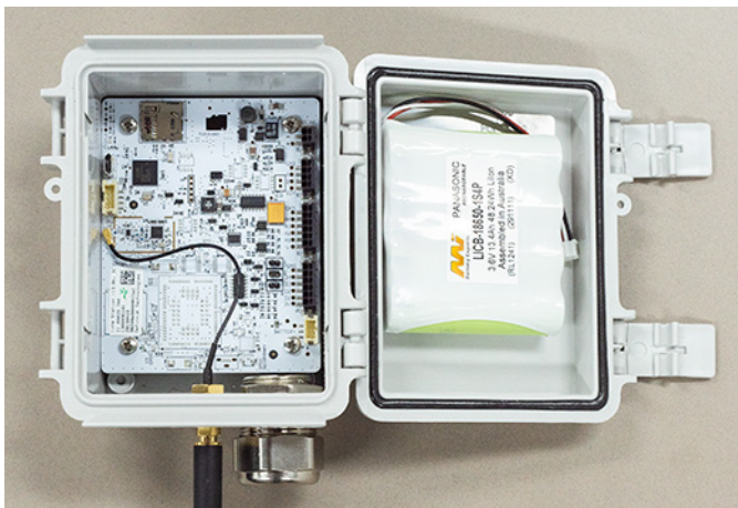
Figure 1. Inside The MFR-Node Box - The MFR-Node Board
