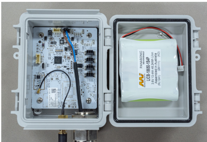
Figure 1. Inside The S-Node Box - The S-Node Board
