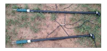
Ensure you have calculated the various poly riser lengths to suit the required depths, factoring how deep they will reach as a complete, buried unit.
