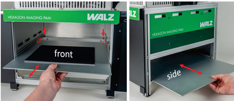
Fig. 6 the supplied base plate can be used in various combinations in the HEXAGON-IMAGING-PAM.
