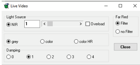
Fig. 24 Selection window for Live Video intensity and color mode – no image saving option.
