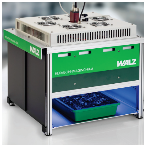
Fig. 3 HEXAGON-IMAGING-PAM seen from the side. The upper bottom plate is taken out. To prevent light from escaping from the side during measurement, the side flaps supplied should be fitted (not shown).
