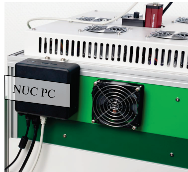
Fig. 2 NUC Windows PC mounted at the side of the HEXAGON-IMAGING-PAM
