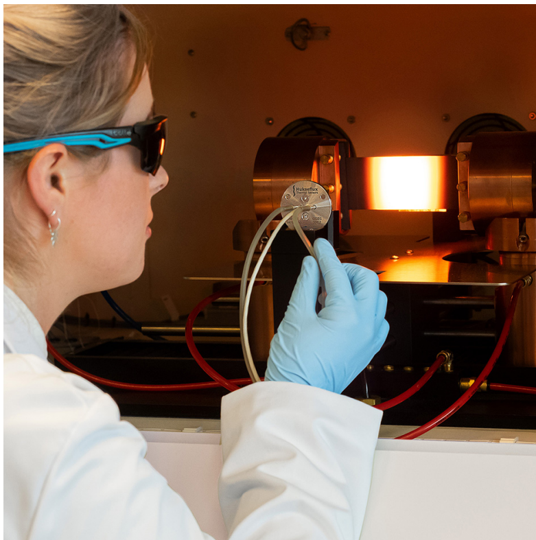
Figure 0.2 GG01 sensor in a high heat flux test cabinet
