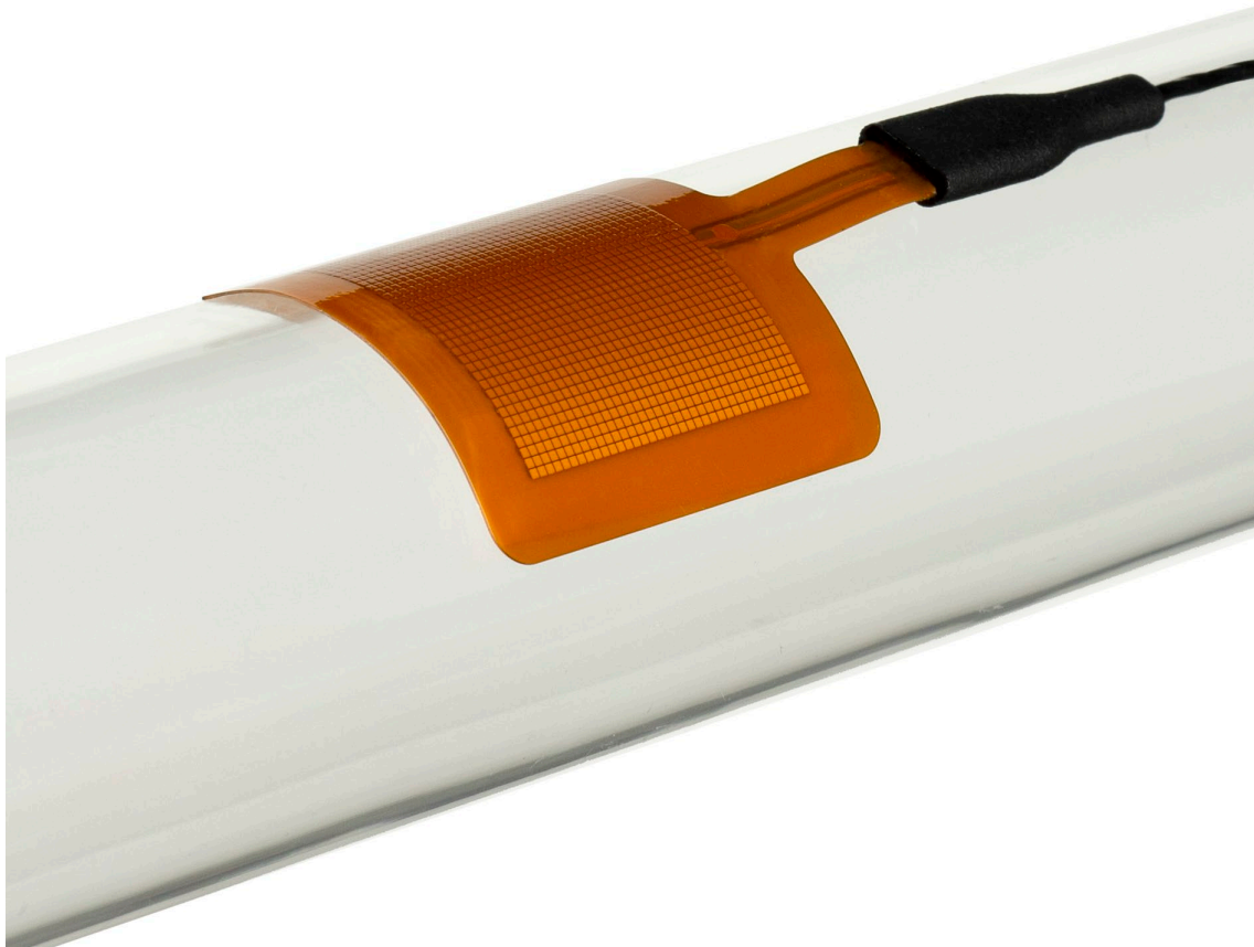
Figure 5.2.1 Bending of model FHF05-50X50 foil heat flux sensor, in this image on a pipe.
