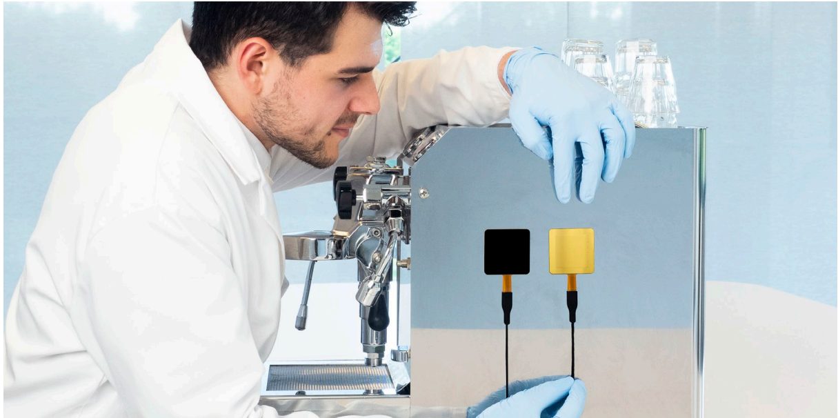
Figure 0.2 Working with BLK - GLD stickers: measuring the radiative and convective heat fluxes on an espresso machine.
