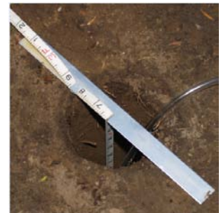
Fig. 17. Tape secured using Tape Holder.
