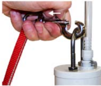
Fig. 13. Connecting Tape Hook to RU.
