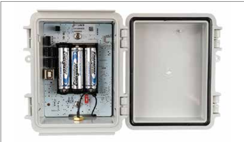
Figure 1. Inside The AD-Node Box - The AD-Node Board
