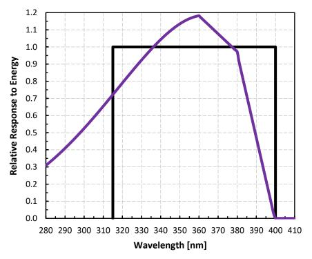
Spectral response estimate of Apogee SU-200 UV-A sensors. Spectral response was modeled from sensitivity of the photodetector and transmittance of the diffuser. Black line shows the UV-A range.
