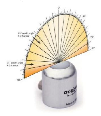
Directional, or cosine, response is defined as the measurement error at a specific angle of radiation incidence. Directional error for Apogee SU-200 series UV-A sensors is approximately  $\pm$  2 % and  $\pm$  5 % at solar zenith angles of 45° and 75°, respectively.
