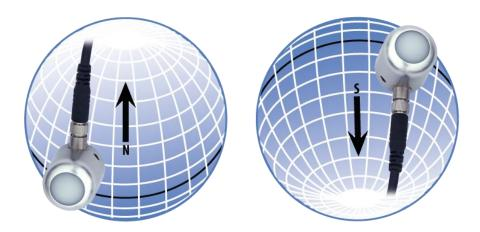
In addition to orienting the cable to point toward the nearest pole, the sensor should also be mounted such that obstructions (e.g., weather station tripod/tower or other instrumentation) do not shade the sensor. **Once mounted, the black cap should be removed from the sensor.** The black cap can be used as a protective covering for the sensor when it is not in use.
