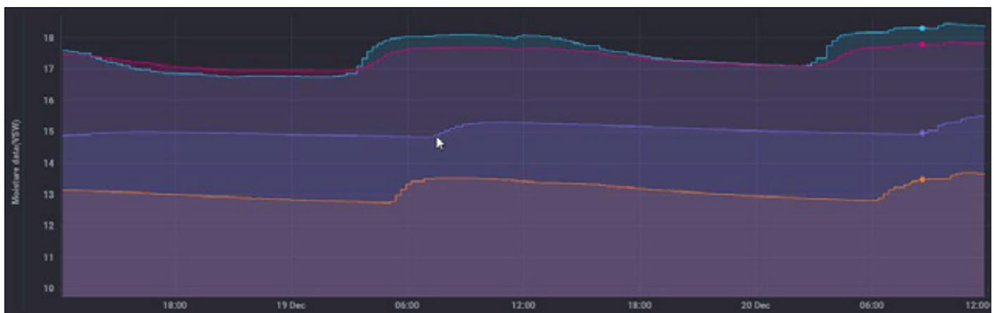
Data from dashboard showing how the MP406 sensors are responding to daily irrigation or rain on the 18th, 19th, 20th December 2019. The Data assisted the park manager with an ability to discern moisture content of selected soil layers (for example 10cm depth) so a decision can be made to judge if the park is under or over-irrigated.
