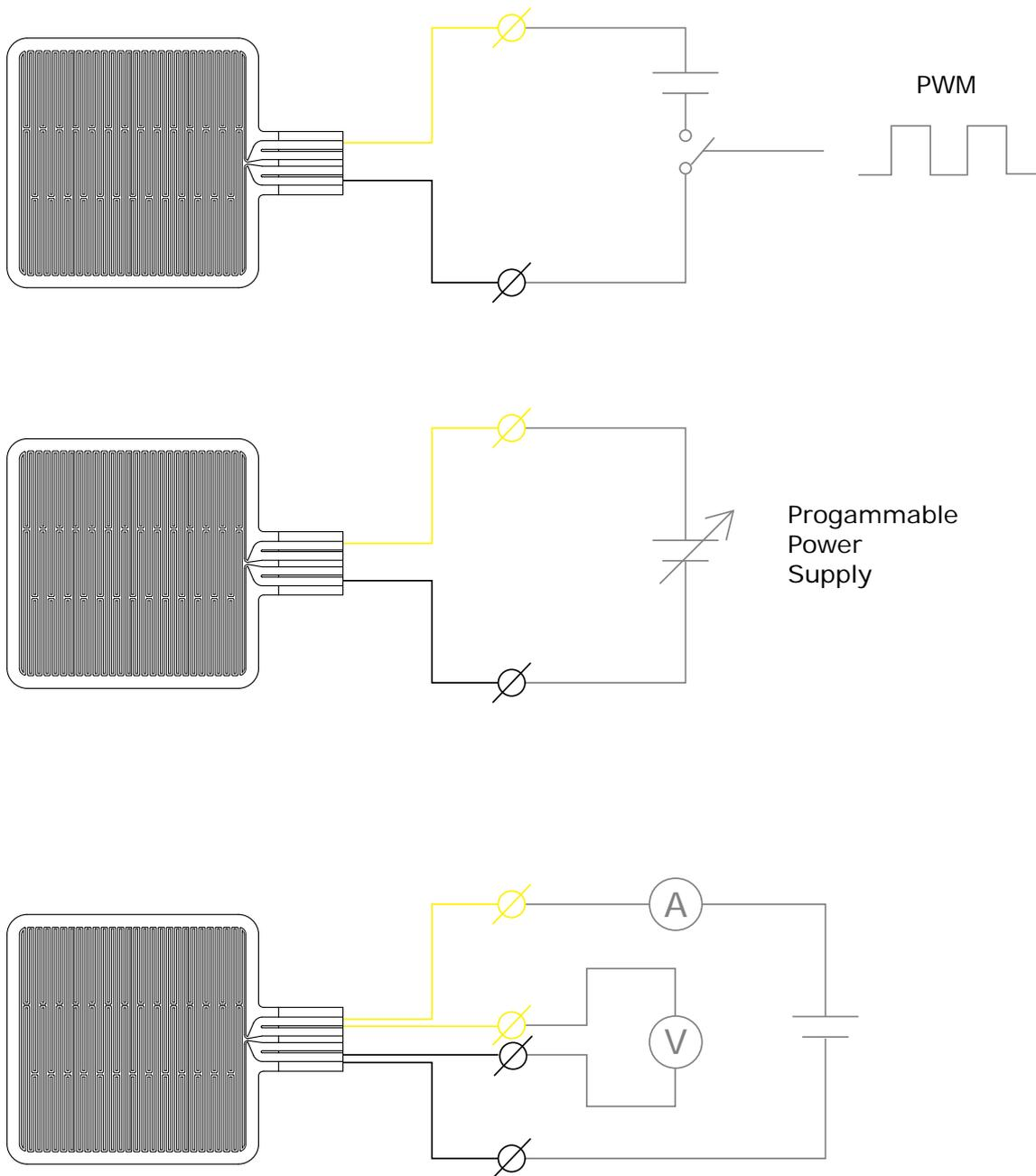
**Figure 4.2.1** Suggested HTR01 heater wiring. Two heater wires are used to carry the heater current; the two others are used to measure the voltage over the heater. There is no significant current flowing through voltage measurement wires so that there is no voltage drop over these wires. This “4-wire connection” measures the true voltage over the heater.
