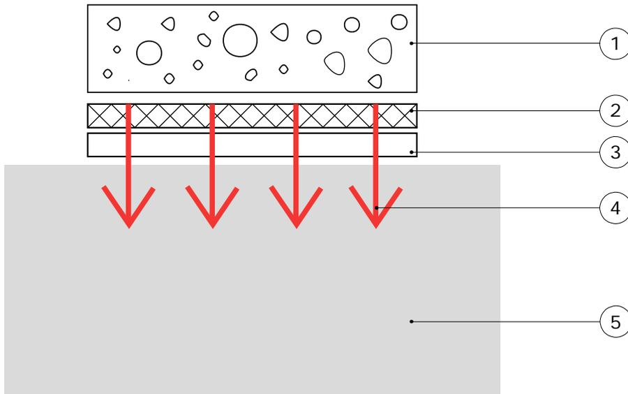
**Figure 2.3.1** Calibration of a heat flux sensor; a typical stack used for calibration consists of a block of metal (mass > 1 kg), for example aluminium (5), the heat flux sensor (3), HTR01 (2) and an insulation foam (1). Under these conditions, heat losses through the insulation are negligible. Heat flux (4) flows from hot to cold.
