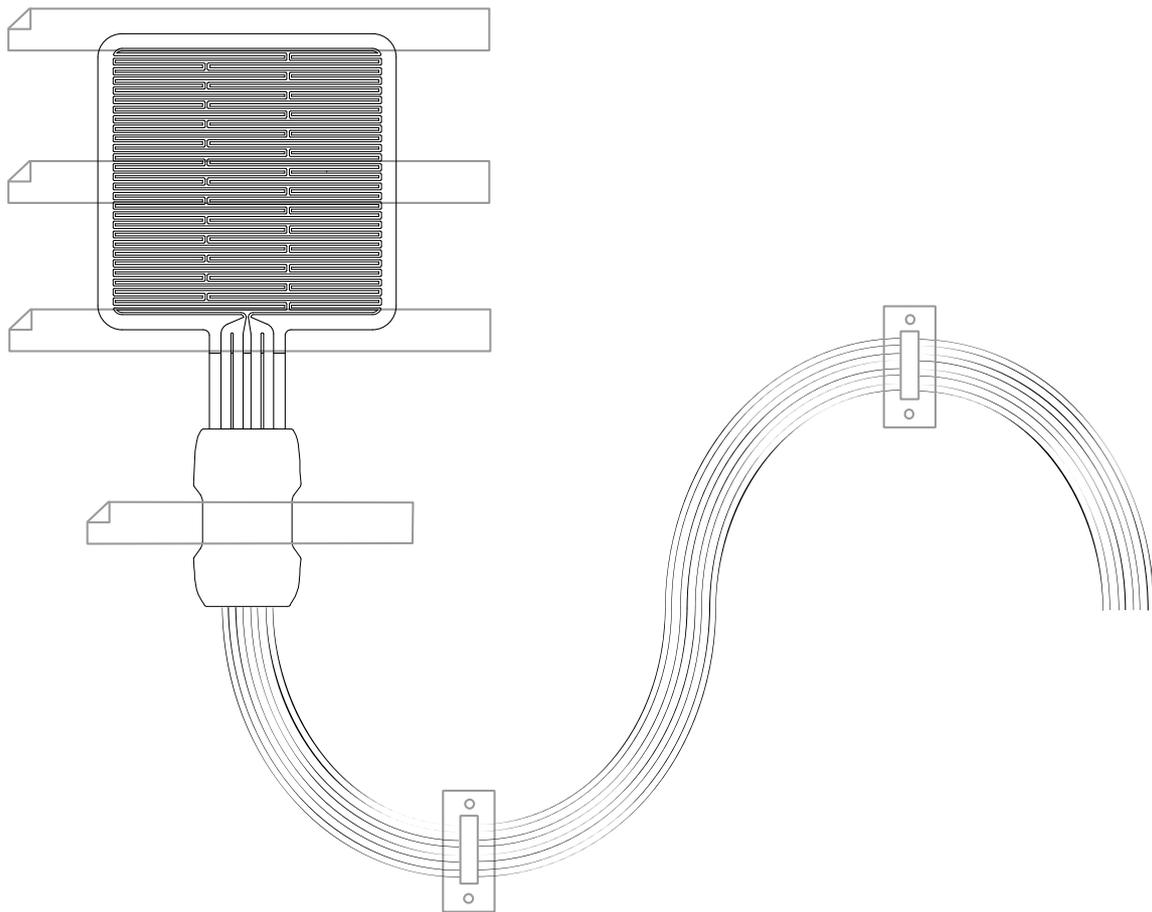
**Figure 4.1.1** *Installation of HTR01 using tape to fixate the sensor and the strain relief block. Extra strain relief of the wire is provided using cable tie mounts equipped with double-sided tape as adhesive. As indicated in Table 4.1.1, tapes fixating the sensor are preferably taped over the passive guard area. In this case, a third tape (in the middle) is added for extra support.*
