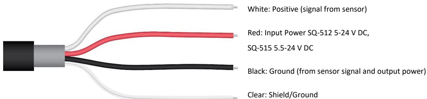
**Wiring for SQ-512 & SQ-515 Serial Numbers within Range 0-1689**
