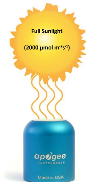
Example of PPFD measurement with an Apogee quantum sensor. Full sunlight yields a PPFD on a horizontal plane at the Earth's surface of approximately  $2000 \mu\text{mol m}^{-2} \text{s}^{-1}$ . This yields an output signal of 2500 mV for the 0-5 V option or an output signal of 1250 mV for the 0-2.5 V option. The signal is converted to PPFD by multiplying by the calibration factor.
