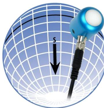
In addition to orienting the cable to point toward the nearest pole, the sensor should also be mounted such that obstructions (e.g., weather station tripod/tower or other instrumentation) do not shade the sensor. **Once mounted, the blue cap should be removed from the sensor.** The blue cap can be used as a protective covering for the sensor when it is not in use.
