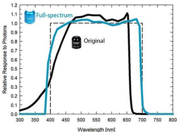
Mean spectral response measurements of six replicate Apogee SQ-100 (original) and SQ-500 (full-spectrum) series quantum sensors. Spectral response measurements were made at 10 nm increments across a wavelength range of 300 to 800 nm with a monochromator and an attached electric light source. Measured spectral data from each quantum sensor were normalized by the measured spectral response of the monochromator/electric light combination, which was measured with a spectroradiometer.
