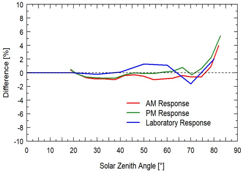
Mean directional (cosine) response of seven apogee SQ-500 series quantum sensors. Directional response measurements were made on the rooftop of the Apogee building in Logan, Utah. Directional response was calculated as the relative difference of SQ-500 quantum sensors from the mean of replicate reference quantum sensors (LI-COR models LI-190 and LI-190R, Kipp & Zonen model PQS 1). Data were also collected in the laboratory using a reference lamp and positioning the sensor at varying angles.
