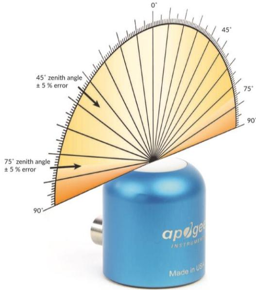
Directional (cosine) response is defined as the measurement error at a specific angle of radiation incidence. Error for Apogee SQ-500 series quantum sensors is approximately ± 2 % and ± 5 % at solar zenith angles of 45° and 75°, respectively.
