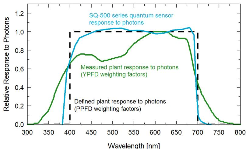
Defined plant response to photons (black line, weighting factors used to calculate PPFD), measured plant response to photons (green line, weighting factors used to calculate YFPD), and SQ-500 series quantum sensor response to photons (sensor spectral response).
