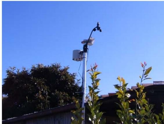
Figure 5: The weather station installed on the site (3.2 m above ground surface)
