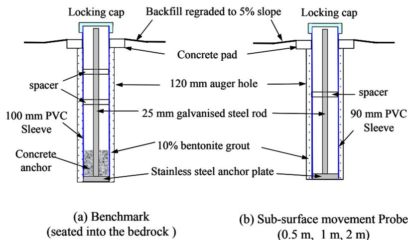
Figure 7: Details of the benchmark and sub-surface movement probes
