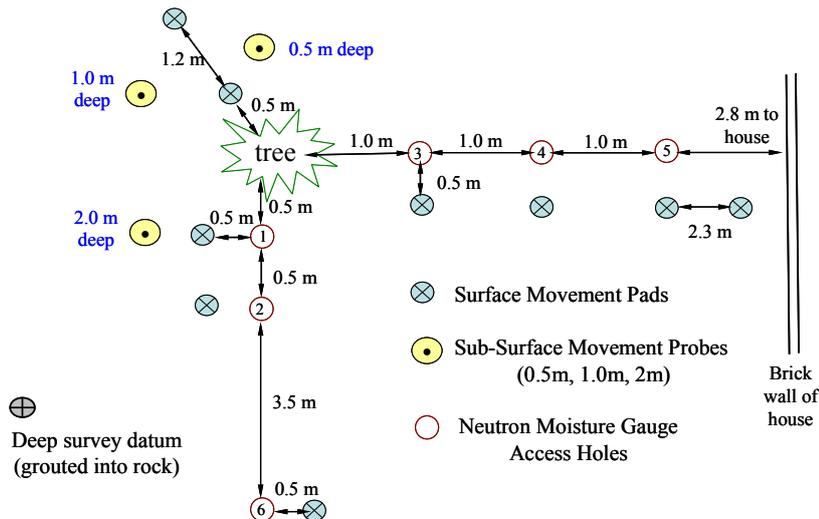
Figure 3: The instrumentation layout at the front yard of the experimental site
