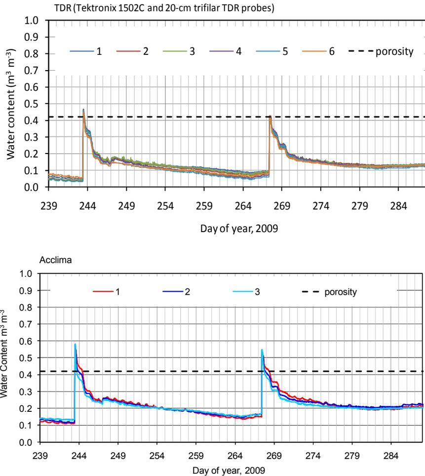
Figure 1. Conventional time domain reflectometry (TDR) water contents using soil-specific calibration (top); and Acclima sensor water contents (bottom).
