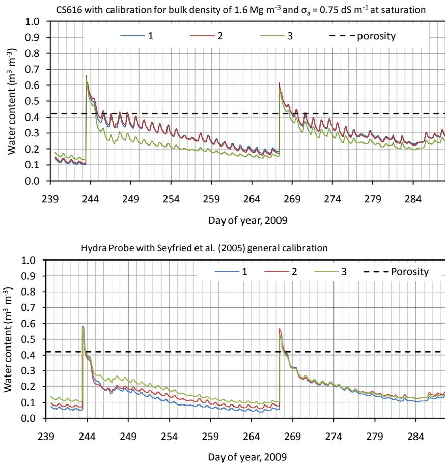
Figure 2. CS616 water contents from calibration for sandy clay loam,  $\rho_b$  of  $1.6 \text{ Mg m}^{-3}$  and  $\sigma_a = 0.75 \text{ dS m}^{-1}$  at saturation (top); and Hydra Probe water contents using Seyfried et al. (2005) general calibration (bottom).
