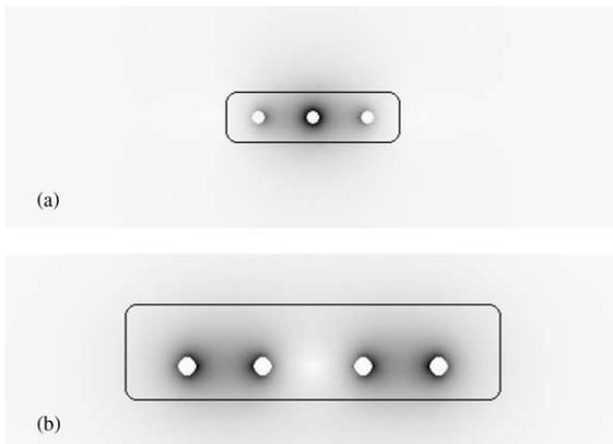
Fig. 4. Cross-sections showing the ATLC (<http://atlc.sourceforge.net/> verified April 14, 2005) (Kirkby, 1996) modeled electromagnetic energy density surrounding probe rods for (a) conventional 3-rod TDR probe with 3.2-mm diameter rods and 12.0-mm rod spacing, and (b) 2-rod Digital TDT Sensor with 4.8-mm diameter rods and 14.2-mm rod spacing.
