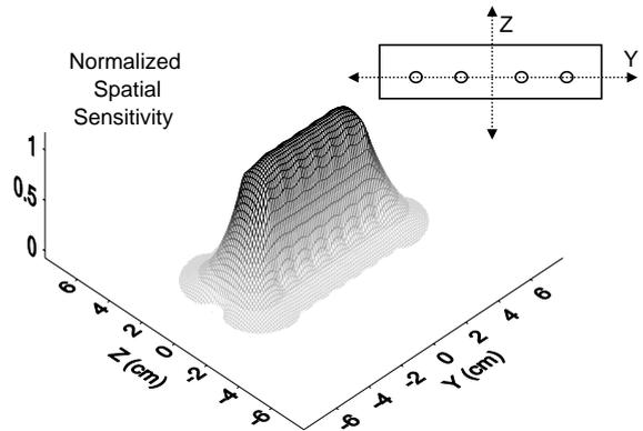
Fig. 5. Three-dimensional plot of the spatial sensitivity of the Digital TDT Sensor in the labeled *y*- and *z*-directions showing the distance from a dielectric discontinuity for which the measurement is no longer influenced by the bordering medium (i.e. normalized spatial sensitivity = 0).
