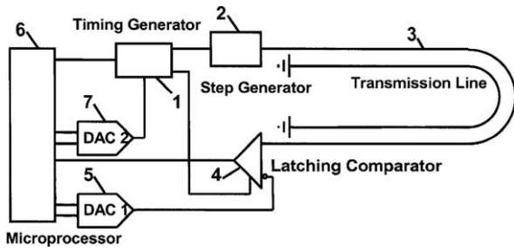
Fig. 2. Schematic drawing of the Acclima Digital TDT Sensor displaying the basic components (Anderson, 2003). The numbers correspond to the following: (1) timing generator; (2) step generator; (3) stainless steel transmission lines; (4) latching comparator; (5) digital to analog converter (DAC) 1; (6) microprocessor; (7) DAC 2.
