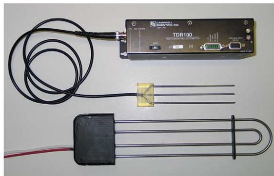
Fig. 1. Photograph comparing the Acclima Digital TDT Sensor and the Campbell Scientific TDR100 connected to a conventional 0.15-m 3-rod probe.
