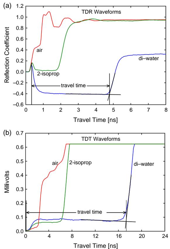
Fig. 3. (a) TDR waveforms in air, de-ionized water, and pure 2-isopropoxyethanol, and (b) TDT waveforms in the same three mediums. The water waveforms display arbitrarily drawn tangent lines to mark the end points from which travel time is measured.
