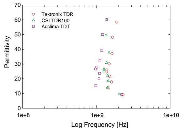
Fig. 7. Maximum passable frequencies of each sensor determined in de-ionized water and 2-isopropoxyethanol mixtures with permittivity values ranging from  $\epsilon \approx 9$ –60.
