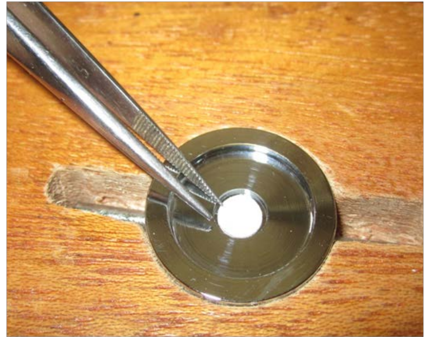
An extracted sap sample on a saturated filter paper being placed into the calibration lid of the PSY1 Stem Psychrometer
