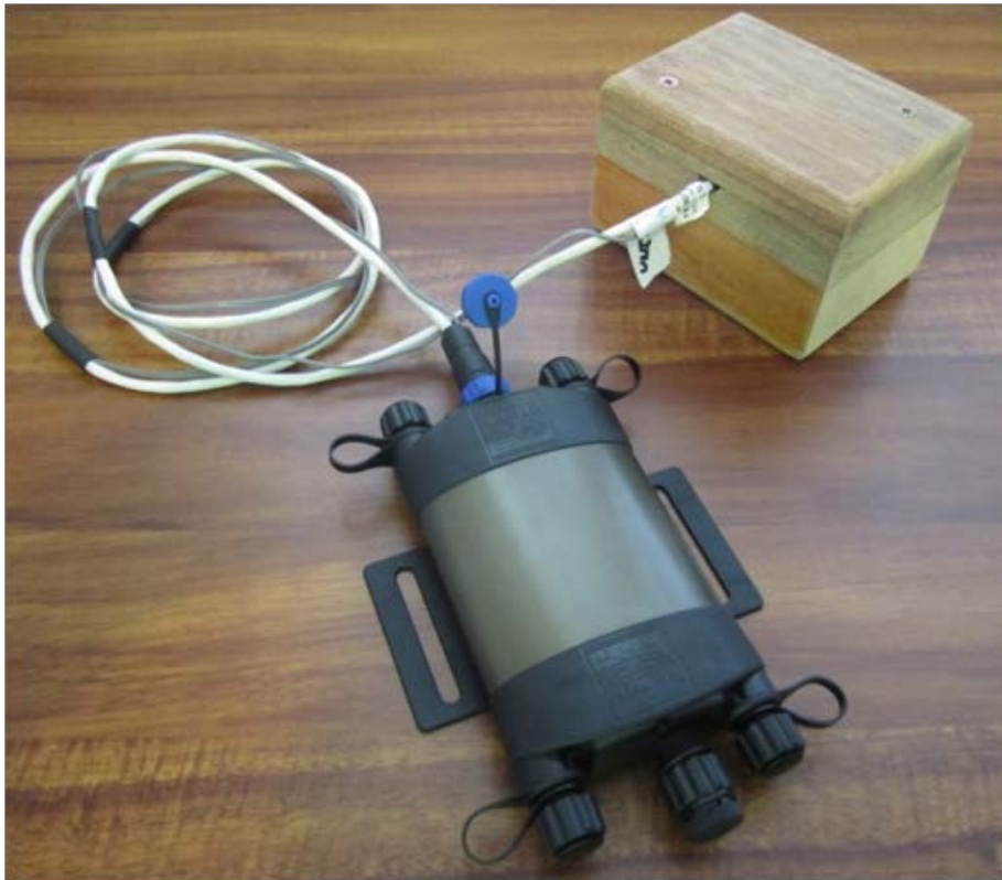
The PSY1 Stem Psychrometer configured for measuring Osmotic potential using the Osmotic Potential Insulator (PSY-OPI)
