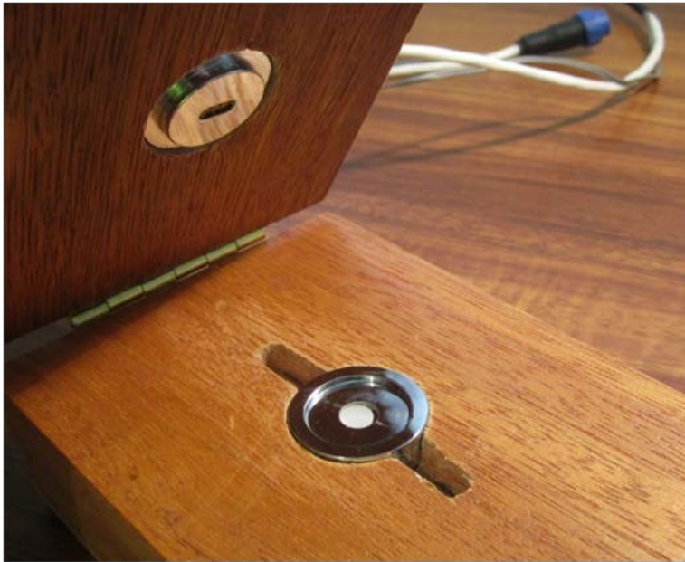
The PSY1 Stem Psychrometer chamber embedded in the Osmotic Potential Insulator.
