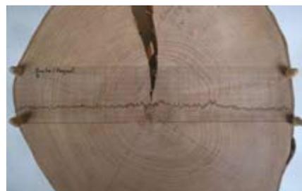
tion to wood density is required to differentiate between intact but soft sapwood and decay.
