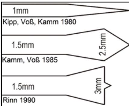
A needle shaft diameter of 1.5mm with a flat tip 3mm wide were found to be a good compromise for achieving maximum resolution and stability, while causing the least damage to the sample.
