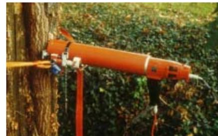
The first series of portable resistance drills were sold to arborists worldwide in 1987. Ehlbeck and Görlacher (1990) proved a linear correlation of its drilling profiles to wood density.
