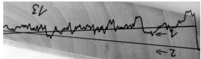
(Left) In diffuse-porous species, such as beech (*Fagus*), tree ring structures can be clearly visible in the profiles due to changes in wood density between earlywood and latewood. But, there can be tree rings where the tree did not build significant latewood layers thus leading to small or even no variations in parts of the profile. Therefore, it is impossible to determine number and width of tree rings.
