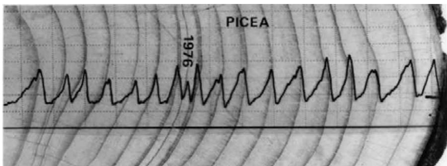
If the needle penetrates the tree rings of conifers radially inward (perpendicular to the stem), the profile clearly reveals differences in density between earlywood and latewood. In this profile of a spruce tree felled in 1986, the extremely dry summer of 1976 can be identified by the correspondingly narrow tree-ring with only a few latewood cells.
