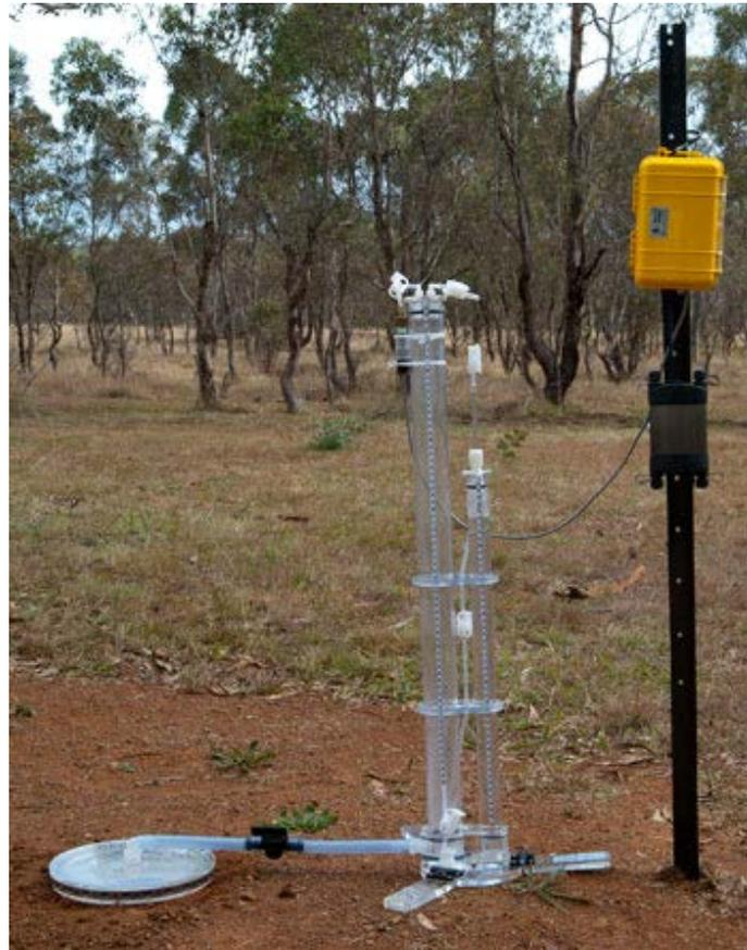
**Photo 1. The AIM Automatic Infiltration Meter consists of a tension infiltrometer, pressure transducer and data logger.**
