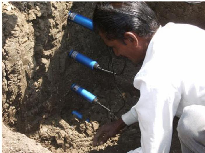
*MP406's installed in a soil profile*
