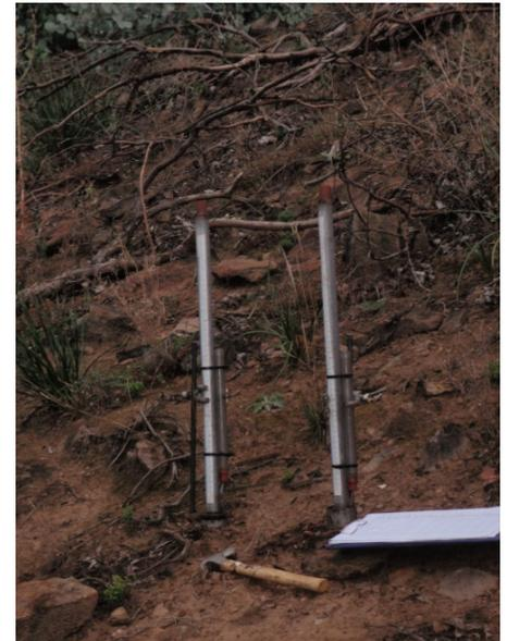
**Figure 4.** Infiltrometers for measuring ponded infiltration rates.
