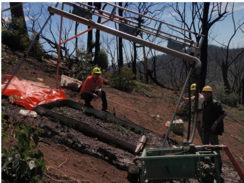
**Figure 5.** Rainfall simulations can only be carried out in areas with easy access, they are expensive and resource intensive but act as a “reality check” for parameters obtained using the mini-disc infiltrometer.
