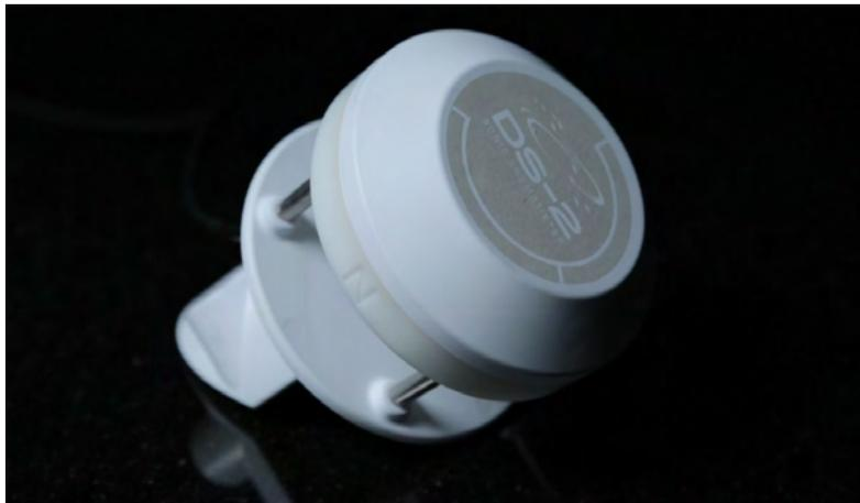
If sampling rate is greater than 0.1 Hz, the anemometer reports the speed and direction at the time of sampling. If sampled less frequently, the anemometer samples every 10 seconds, averages the vector components of the wind, and keeps the maximum gust. When the logger samples, the anemometer reports the average wind speed, direction, and the maximum gust speed.
