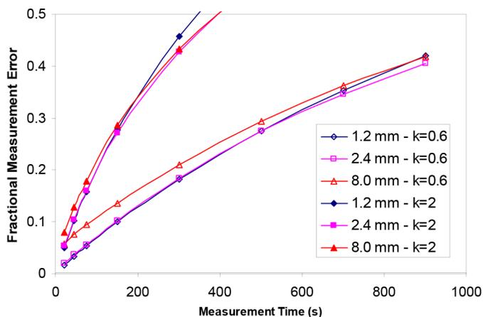
Figure 2. Error in computing  $k$  as a function of time of slope measurement for the probes in Table 1 when the temperature drift in the material under test is 0.001 C/s for two thermal conductivities.
