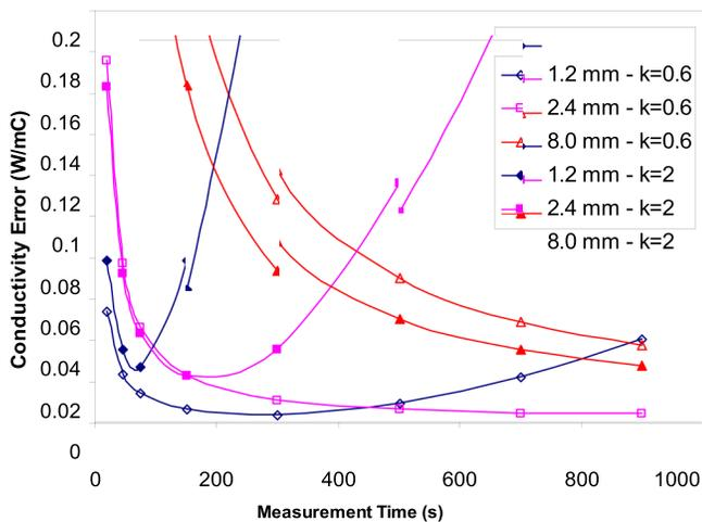
Figure 1. Error in the  $k$  value computed using eq. 4 as a function of the time at which the slope is computed for the probes shown in Table 1. This information is for uncalibrated probes. Properties for the simulation are moist soil and saturated quartz sand.
