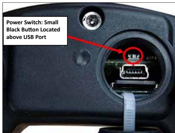
Picture above: the PSY1 can also be automatically powered up by connecting it to a power supply. This can either be in the form of a Mains to 24 volt DC power supply, a solar panel, USB connection or external 12V battery. (See Charging - Powering the Instrument in the PSY1 manual).
