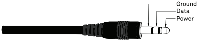
Figure 1 3.5-mm stereo plug connector wiring
