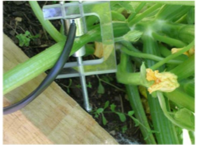
Installation of Stem Psychrometer
