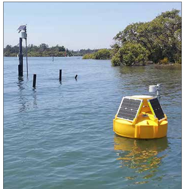
CATM1-based water quality monitoring Data Buoy located at mid-north coast, NSW Australia.
