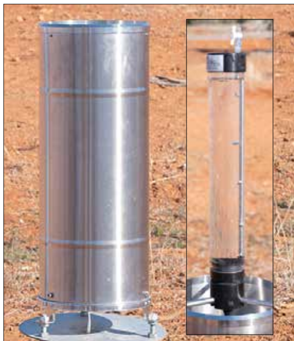
Figure of Tipping Bucket Rain Gauge Calibration TBRG Field Kit In Use on an ICT International SRG0
