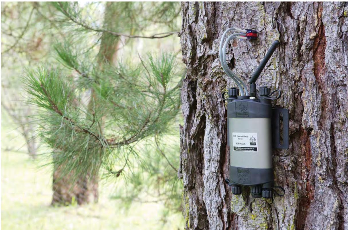
Photo 4: SFM1 Sap Flow Meter Installed on a *Pinus radiata* tree.
