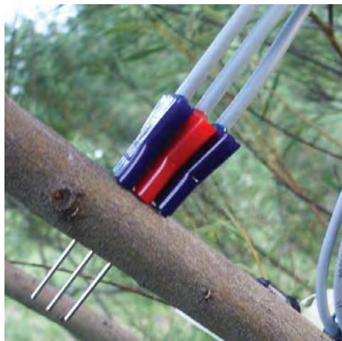
Photo 2: SFM1 Measurement Needle Set installed in a small diameter woody stem or branch.
