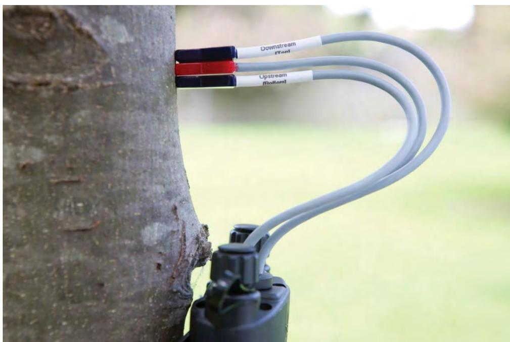
Photo 3: Colour coded and labelled SFM1 needles.
