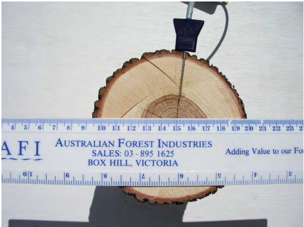
Photo 48: Measuring the Stem Diameter and sapwood depth of Callitris glaucophylla .
