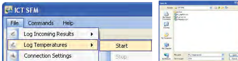
Figure 105: Start Log Temperatures function to record raw temperatures to a file on the computer.
