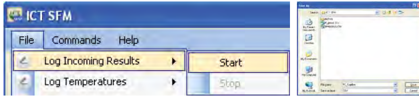
Figure 101: The Menu sequence required to start Logging Incoming Sap Flow data direct to the computer.
