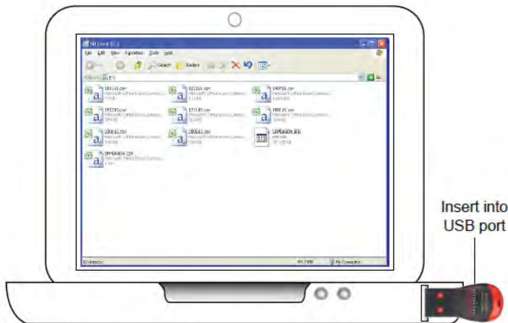
Figure 98: MicroSD Card Adaptor with the MicroSD card from the SFM1 inserted into the USB port of a computer.
