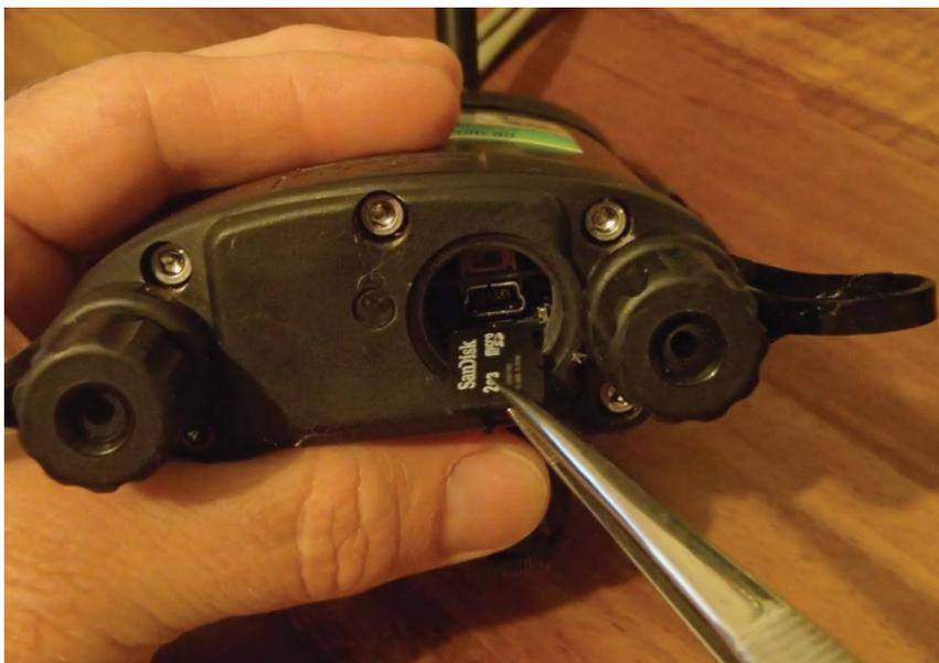
Photo 45: Removing the MicroSD card using a pair of forceps (tweezers) via the communications port.
