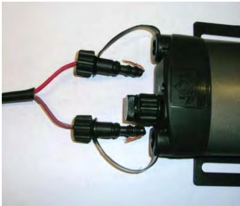
Photo 13: Inserting the power-bus plugs with stripped cable into the power bus ports on either side of the SFM1
