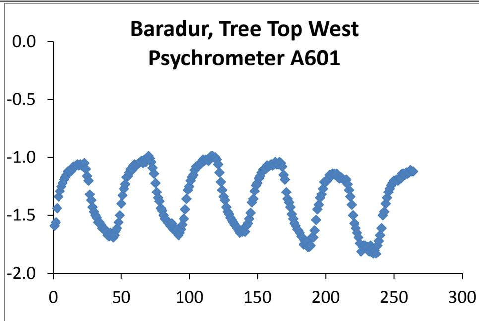
**Figure 1 - 5 daily cycles of water potential measured with ICT psychrometer on a branch at about 88 meter height in a 91 meter tall *Sequoiadendron giganteum* At Whitaker’s Forest, California during the period Aug. 13 – Aug. 17, 2010. Unpublished Data - Courtesy George Koch Northern Arizona University**
