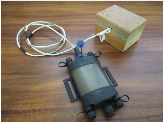
The psychrometer chamber is housed in the Osmotic Potential Insulator (OPI) to provide a thermal insulating jacket around the chamber. This eliminates introduction of thermal gradients caused by a need to handle the chamber to load samples and provides a stable insulated thermal buffer from ambient temperature gradients within the surrounding environment. This enables a very rapid equilibration time between samples.
