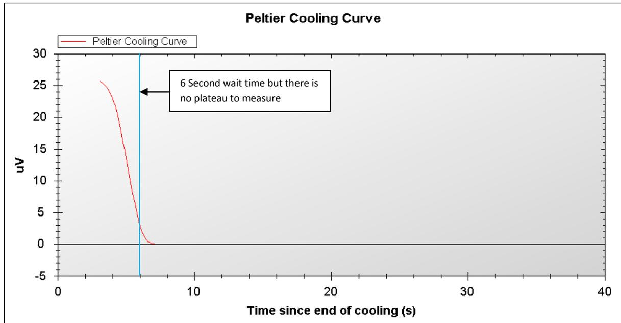
**Figure 27: Peltier cooling curve with insufficient cooling time.**
