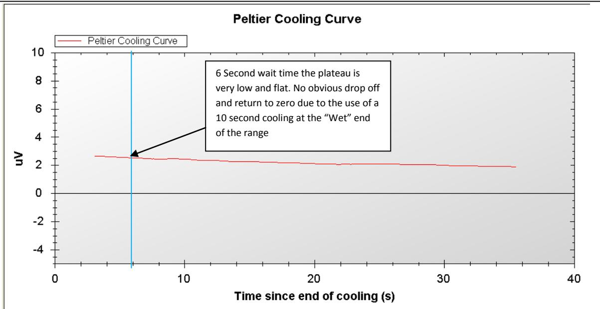
**Figure 28: Peltier cooling curve with an excessive cooling time relative to the water potential of the sample resulting in a much longer time required for Thermocouple-C to return to zero reference. This sample was taken on *Sequoia sempervirens* (Coast Redwood) and the measured water potential (-0.76 MPa) was simultaneously verified against a Scholander pressure bomb (-0.73MPa)**
