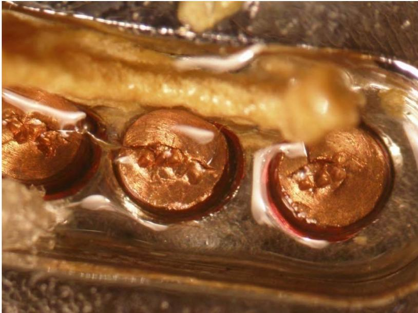
**Photo 9:** A heavily contaminated stem psychrometer in which the chamber well has been filled with vacuum grease and plant tissue or callus, this type of contamination is clearly obvious from visual observation.
