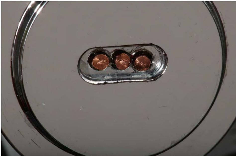
Photo 15: The corresponding psychrometer that generated the Peltier cooling curve in Figure 6. Note there is no visually obvious dirt or contamination. This is why it is important to clean and test with a 1.0 Molal NaCl solution before deployment
