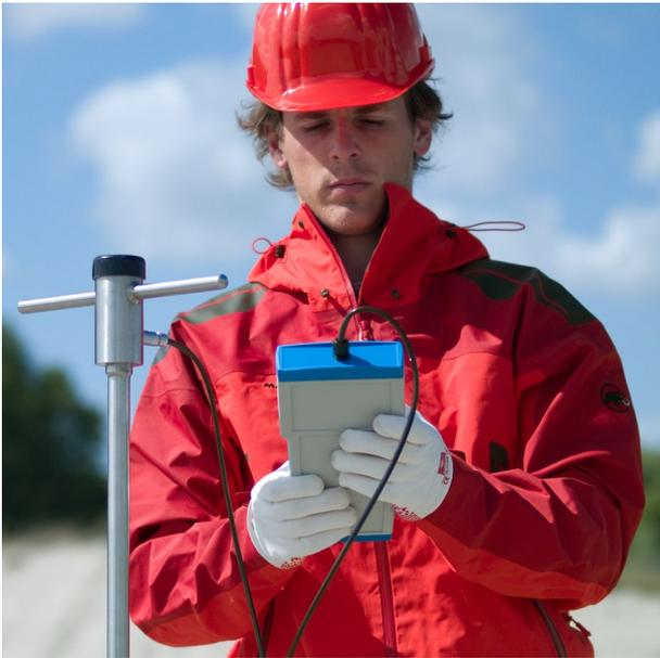
**Figure 1** Soil thermal route survey with FTN01 including CRU01 control and readout unit
