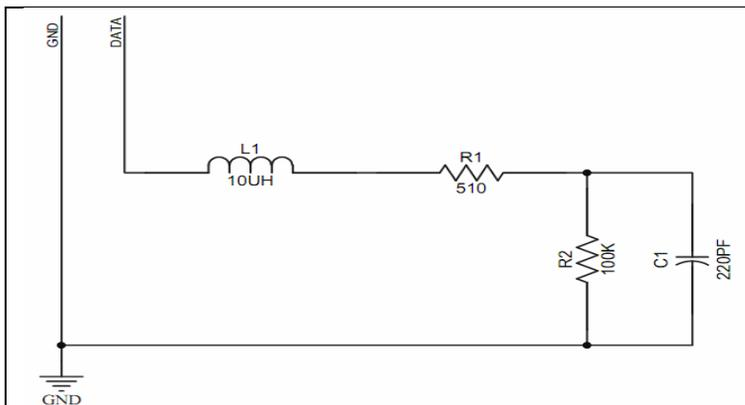
**NOTE:** This is a low impedance variant of the recommended SDI-12 Specification. This allows up to 62 sensors to be maintained on a bus.
