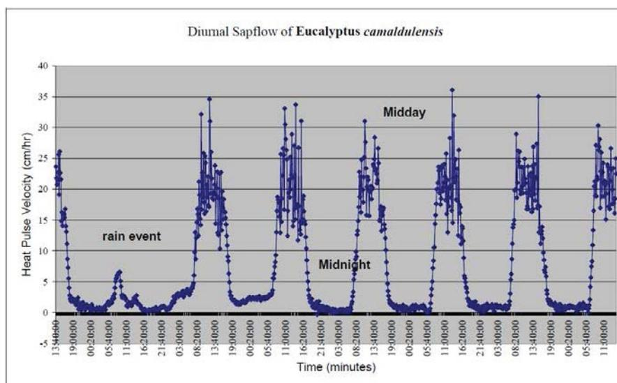
Figure 119 shows a typical diurnal heat pulse velocity pattern of a *Eucalyptus camaldulensis* with very 'clean' HRM data with no obvious problems, with needles well in conducting sapwood over a period of 1 week. Zero flows are experienced at night time with fluctuating peaks throughout the day in response to changing light conditions and evaporative demand. In this example the effect of a rainfall event on sap flow can be clearly seen.
