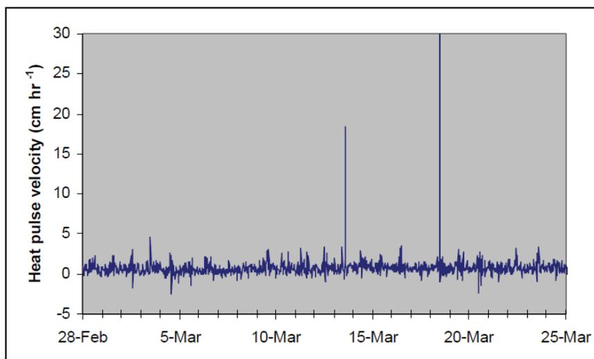
Figure 120 Data from probes installed in wood with poor hydraulic conductance: This is typically what you might see if these TC junctions were located in non-conducting heartwood or cambium/bark tissue. There is only a very slight diurnal pattern of heat pulse velocity (HPV). Note also that minimum HPV is very well aligned with the zero line, indicating that probe alignment in this example was quite good, assuming there was next to zero sap flow at this measurement point.
