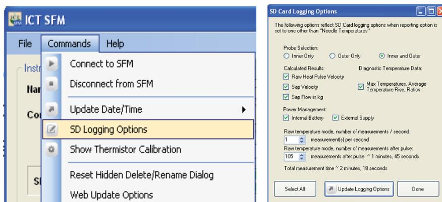
Figure 86 The SD Card Logging Options tab showing that the calculated parameters of Raw Heat Pulse Velocity, Sap Velocity and Sap Flow will be logged to the \*.CSV data file along with the Diagnostic Temperature data Max Temperature, Average Temperature Rise, Ratios and Power management data; internal battery and External Supply.
